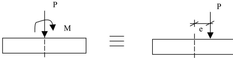
Fig. 8.3 Moment as Equivalent to Eccentric Axial Load
