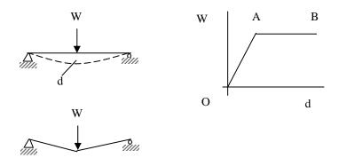
In general, the bending moment along a beam is not uniform and in the centrally-loaded beam, the maximum moment occurs at a single cross-section. If the load-point deflection d is recorded while the load W increases from zero, the initial behaviour will be elastic to give the straight line OA. When the maximum moment reaches the fully plastic moment, a very large curvature is now possible and the deflection increases with no change in load (i.e. A to B).
