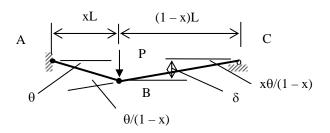
Work done by external load =  $P\delta$ Work done in hinges = Work done in hinge at A + Work done in hinge at B
