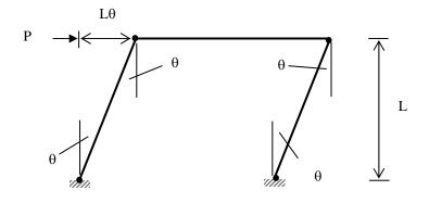
Using the same virtual work procedure as for the beam mechanism, and noting that all members are of the same section,
