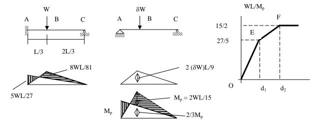
As long as the beam remains elastic, normal elastic analysis gives the bending moment diagram, which is shown on the left via the superimposition method of presenting BMDs.
