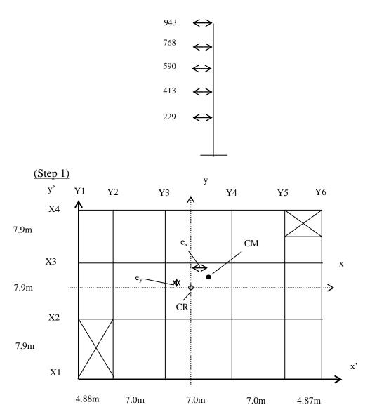
The  $x_i$ , (for the Y frames) are: 0,4.88, 11.88, 18.88, 25.88, 30.75 m The  $y_i$  (for the X frames) are: 0, 7.9, 15.8, 23.7m
