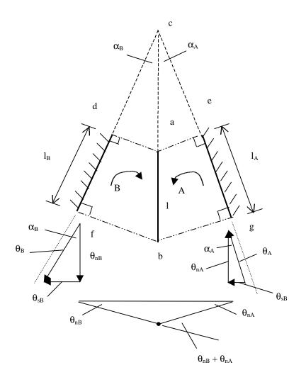
The yield line ab divides the slab portion dfbgea into the two rigid portions A and B. A rotates  $\theta_A$  about support axis eg and B rotates  $\theta_B$  about support axis df. The rotations are represented by vectors following the right-hand-corkscrew rule.
