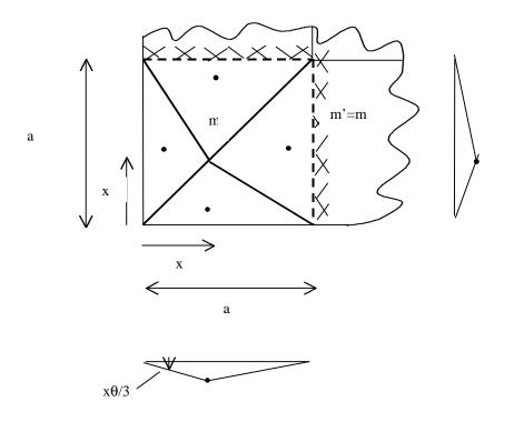
Work done by the external loads is the sum of the load through the centroid of each rigid region, times the deflection of the rigid region at the centroid.
