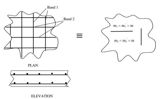
For isotropically reinforced slabs, the reinforcement is usually parallel (and perpendicular) to the predominant support line. Also, in the conventional notation, the m lines, called the *moment axes*, are perpendicular to the reinforcement, as shown above.
