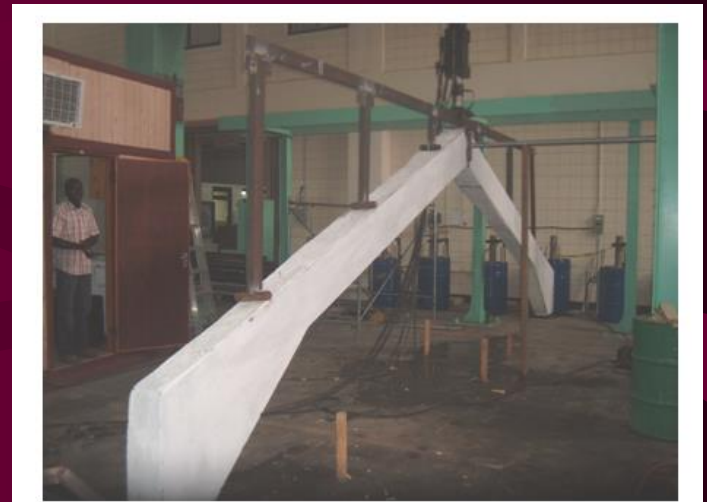
Figure 6. Photograph of test setup for ferrocement pitched portal frame
