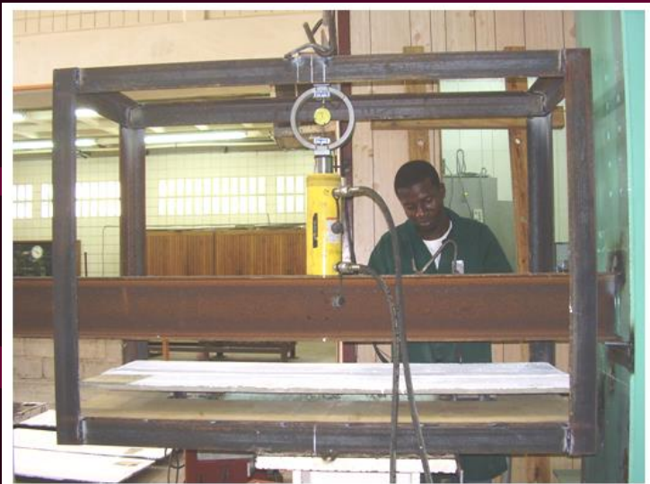
Figure 11. Photograph of pullout testing of roof slab-to-beam connection
