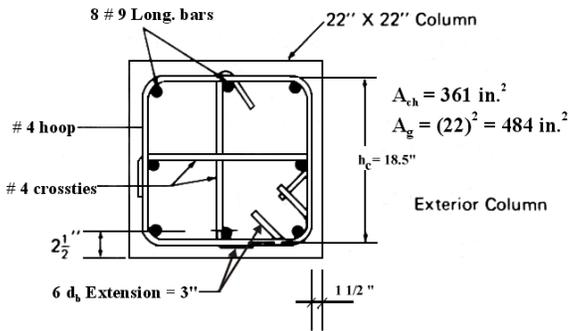
Figure 10-58. Detail of column transverse reinforcement.
