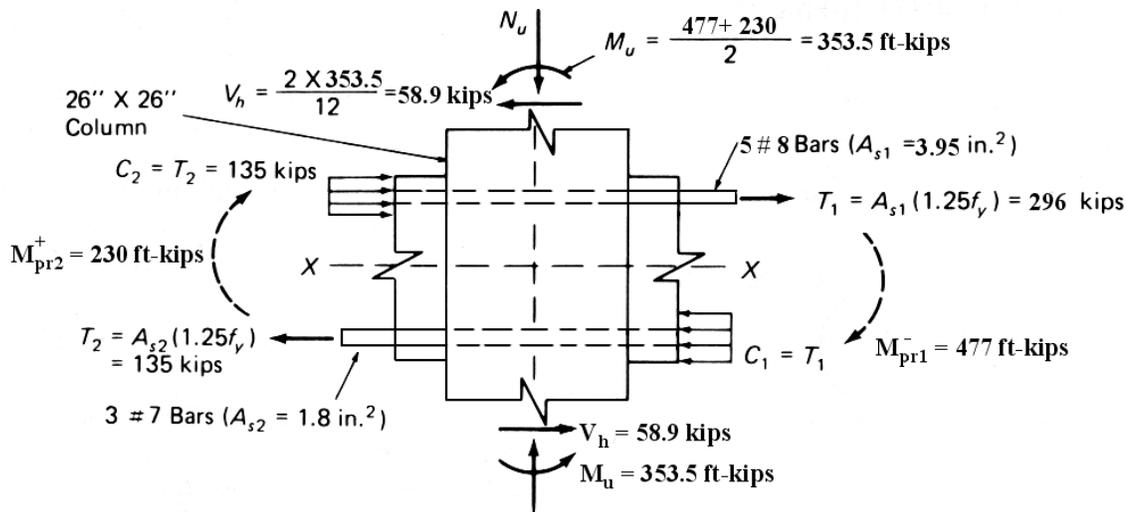
Figure 10-62. Forces acting on interior beam-column joint.
