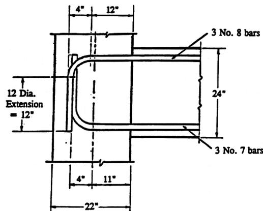
Figure 10-52. Detail of anchorage of flexural reinforcement in exterior column
