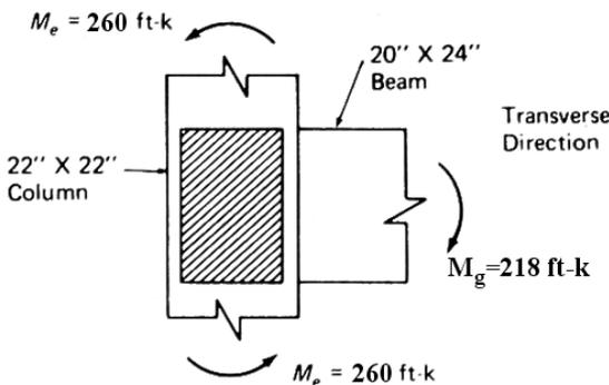
Figure 10-56. Relative flexural strength of beam and columns at exterior joint—transverse direction.
