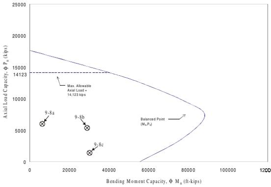
Figure 10-63. Axial load-moment interaction diagram for structural wall section.
