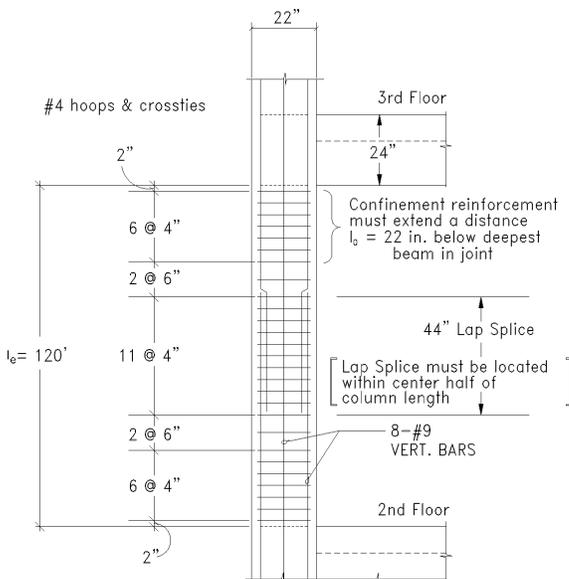
Figure 10-59. Column reinforcement details.
