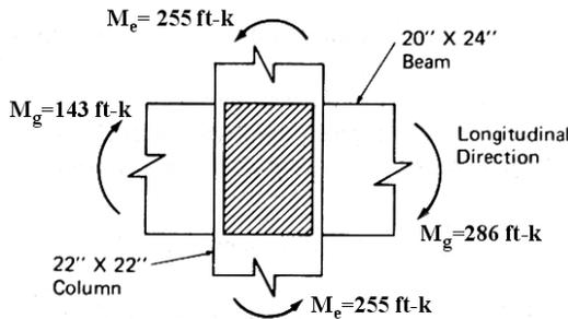
Figure 10-57. Relative flexural strength of beam and columns at exterior joint—longitudinal direction.
