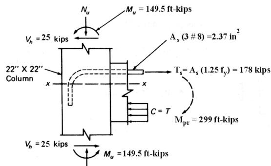
Figure 10-60. Horizontal shear in exterior beam-column joint.
