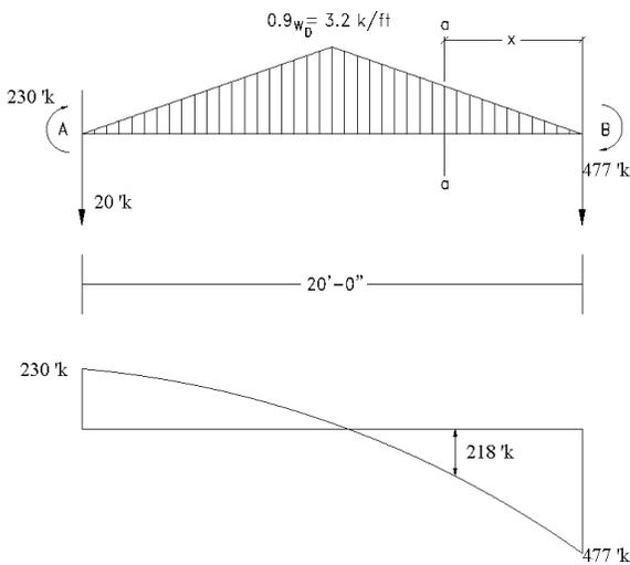
Figure 10-54. Moment diagram for beam AB
