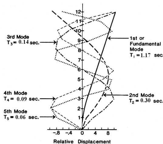
Figure 10-49. Undamped natural modes and periods of vibration of structure in transverse direction
