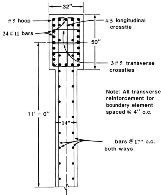
Figure 10-64. Half section of structural wall at base.
