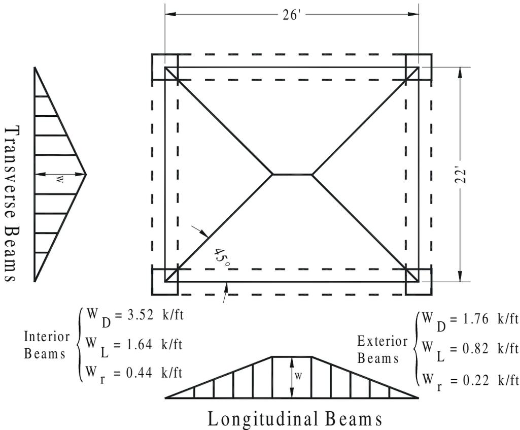
Figure 10-51. Tributary area for beam loading.
