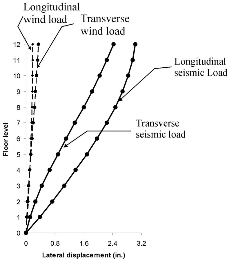
Figure 10-50. Lateral displacements under seismic and wind loads.
