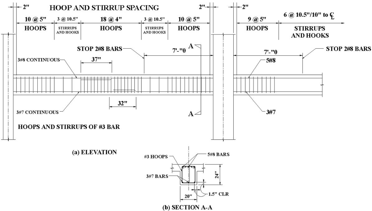
Figure 10-55. Detail of reinforcement for beam AB.
