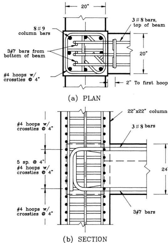
Figure 10-61. Detail of exterior beam-column connection.
