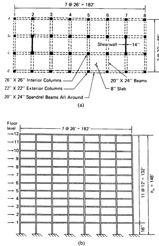
Figure 10-48. Structure considered in design example. (a) Typical floor framing plan. (b) Longitudinal section
