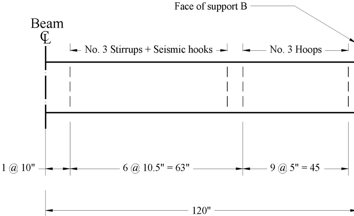
Figure 10-53. Spacing of hoops and stirrups in right half of beam AB
